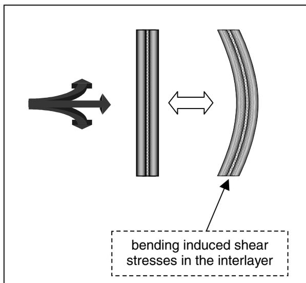
The vibration damping effect of an acoustic PVB is easily visualized in a relatively simple experiment: A laminated bar carrying a small accelerometer is excited with a short strike to freely vibrate on two foam supports. The difference in terms of the decay of the amplitudes between a standard PVB and an acoustic PVB is obvious (see figure 3).
