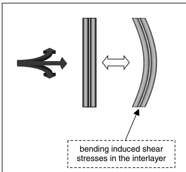
The vibration damping effect of an acoustic PVB is easily visualized in a relatively simple experiment: A laminated bar carrying a small accelerometer is excited with a short strike to freely vibrate on two foam supports. The difference in terms of the decay of the amplitudes between a standard PVB and an acoustic PVB is obvious (see figure 3).
