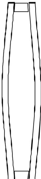
Figure 4. Section through a sealed insulating glass unit with high internal air space pressure. (exaggerated horizontal scale).
