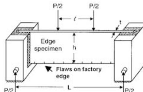
Figure 2. Four-point bend fixture for measuring edge strength
