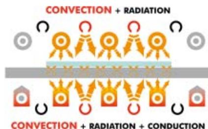
Picture 4. Profiled high convection heating system (Tamglass patent).
