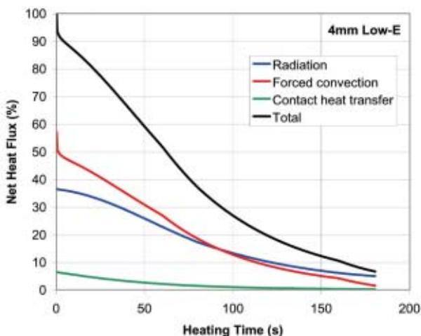
There are two methods to apply forced convection heating on the market. The traditional closed circulation high volume convection method with blowers and nozzle system inside the furnace and the latest profiled high speed convection method with filtered and compressed air jets.
