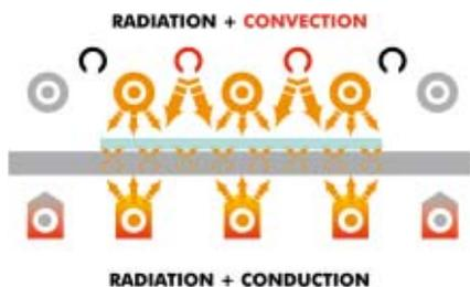
Picture 3. Longitudinal profiled top convection/radiation system (Tamglass patent).
